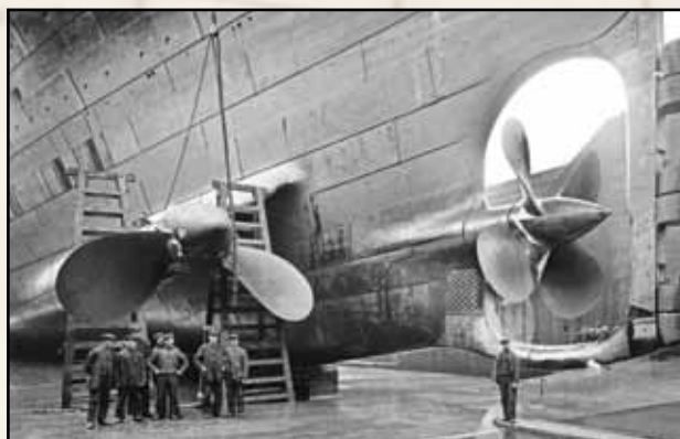
Olympic centre propeller and port propeller with missing blade, Thompson Graving Dock with posed workers, March 1912.
